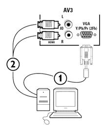
You may connect your computer to the **VGA** connector of **AV3** or to the **HDMI** connector (see further).
