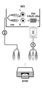
Connect the device with **2Fh YPbPr** output to the **VGA** connector (1) (with the supplied adapter cable VGA to cinch) and to the **L** and **R AUDIO** jacks (2) of **AV3**. See also the manual of your High Definition device.
