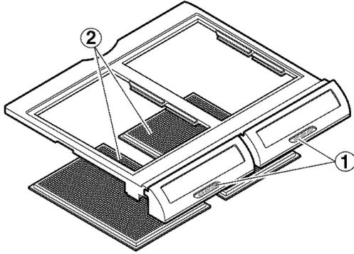
The Optibin Crisppers provide fresher-tasting fruit and vegetables by letting you easily control humidity inside the crisper. The Optibin Crisppers include: 1) a humidity control knob at the front of the crisper cover and 2) a large lattice on the inner surface of the cover to hold or release moisture.
