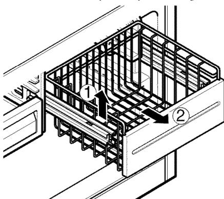
2. To Install, pull both rails out to full extension. Hook the basket supports into the rail tabs and push to the back of compartment.
