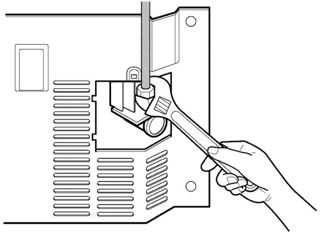
5. Bend the pipe to upwards and replace the cover into original position. And tighten the screw.
