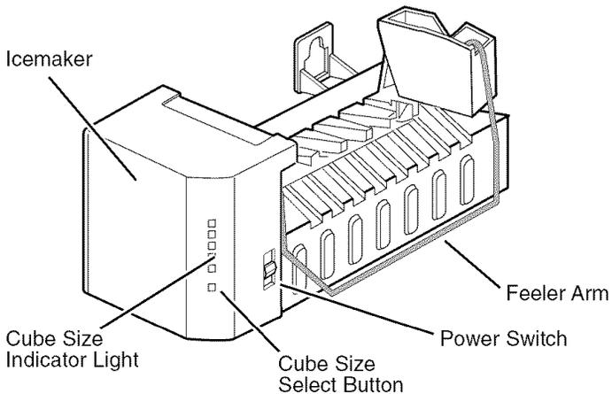
The icemaker will produce eight cubes per cycle—approximately 100–130 cubes in a 24-hour period, depending on freezer compartment temperature, room temperature, number of door openings and other operating conditions.
