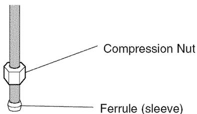
4. Insert the pipe into the valve and fasten with spanner as shown in the figure below.
