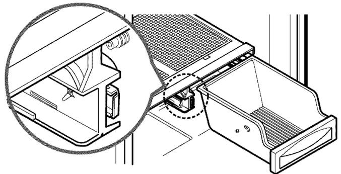
3. Slightly tilt up the front and push back until it snaps into place.
