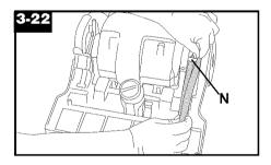
With lettering to the outside of belt, slide new belt along side of cleaner cavity and over motor pulley (N).
