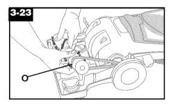
Insert agitator through belt and place belt in belt guide (O).
