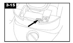
Pull old bulb straight out of socket. Push new bulb straight into socket until locked in place.
