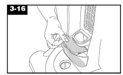
Snap access door into place. Reposition dirt cup (Fig. 3-10).
