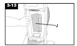
Lift out filter (J) and hand wash in cold water with a mild detergent.
