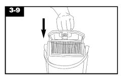
Replace lid and filter on filter chamber. Replace chamber on dirt cup.
