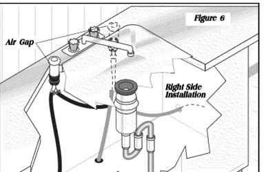
3. If you connect to a sink trap, local codes may require you to install an air gap kit, not included. The drain hose will be routed from dishwasher to air gap inlet as shown in Figure 6. An air gap kit is available from a plumbing supply store.
