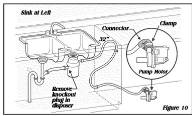
The drain hose loop must be at least 32" high from the floor to insure proper drainage.
