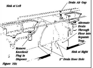
5. Before cutting drain hose access, check both sides of selected area to avoid interference. Cut a 2" diameter hole in shaded area shown in Figure 2.
