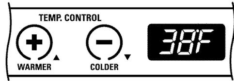
**To change the temperature setting**, press the WARMER or COLDER pads until you reach the desired set temperature. After several seconds, the display will return to the actual temperature.
