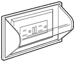
**Refrigerator MUST be plugged into a functioning GFCI circuit.** Test your circuit by plugging your refrigerator into the outlet and pressing the test button for that circuit, verifying that the unit turns off (the light will not work with the door open). Then press the Reset button and confirm that the light comes on with the door open. If you do not know if you have a GFCI circuit, contact a qualified electrician for assistance.
