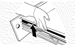
Open the drawer fully. Using the finger grasp holds on the side of the drawer, lift the pan up and out.
