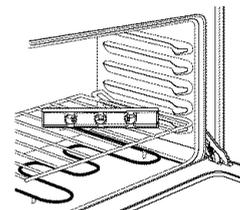
**B** Turn the legs clockwise to raise the range and counterclockwise to lower the range. Adjust the leveling legs until the range is level.
