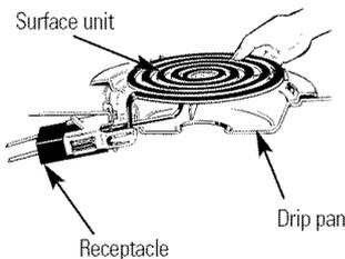
To remove the surface unit, lift it about 1 inch above the drip pan and pull it out.
