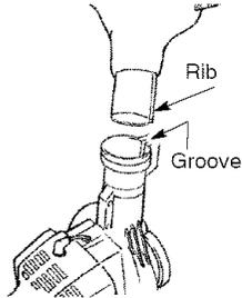
5. Insert the elbow tube into the blower outlet. Make sure elbow tube is aligned with the blower outlet groove.
