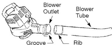
2. Secure the tube by turning the knob clockwise.
