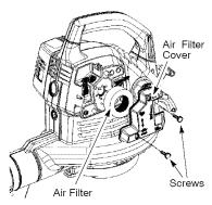
A dirty air filter decreases engine performance and increases fuel consumption and harmful emissions. Always clean after every 5 hours of operation.
