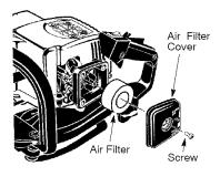
A dirty air filter decreases engine performance and increases fuel consumption and harmful emissions. Always clean after every 5 hours of operation.
