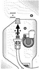
3. Place brass nut (A) and sleeve (B) on copper tube end as illustrated. (Do not use old sleeve.)
