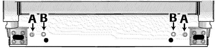
5. Using the carpenter's level, make sure front of refrigerator is 1/4" (6 mm) or 1/2 bubble higher than back of refrigerator and that the refrigerator is level from side to side.
