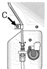
7. Monitor water connection for 24 hours. Correct leaks, if necessary.
