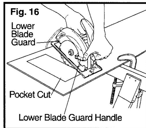
**⚠ WARNING: NEVER** tie the lower blade guard in the raised position. Leaving the blade exposed could result in serious injury.
