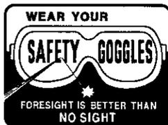
**⚠ WARNING:** The operation of any circular saw can result in foreign objects being thrown into your eyes, which can result in severe eye damage. Before beginning power tool operation, **ALWAYS** wear safety goggles or safety glasses with side shield and a full face shield when needed. We recommend A Wide Vision Safety Mask for use over eyeglasses or standard safety glasses with side shield, available at Sears Retail Stores.
