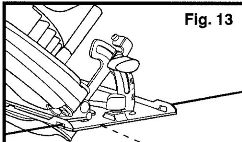
Align Inner Blade Guide Notch on Shoe with Line of Cut (as shown) When Making  $45^{\circ}$  Bevel Cuts
