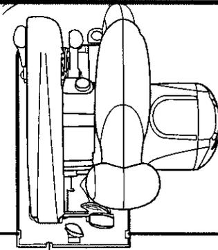
Align Outer Blade Guide Notch on Saw Base with Line of Cut (as shown) When Making Cross Cuts or Rip Cuts
