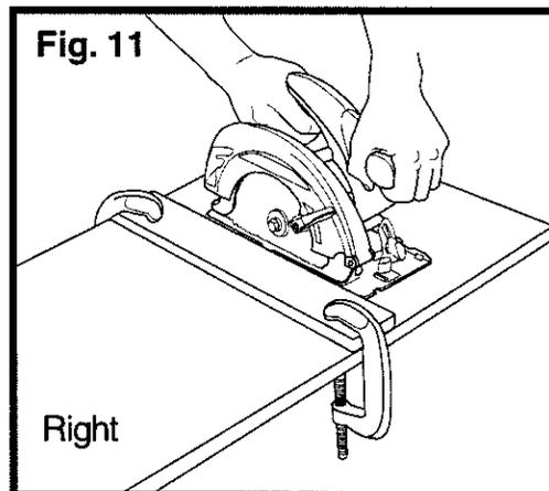
**⚠ WARNING:** If the blade comes in contact with the workpiece before it reaches full speed, it could cause the saw to kickback towards you, resulting in serious injury.
