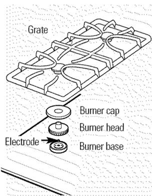
**CAUTION:** DO NOT OPERATE THE BURNER WITHOUT ALL BURNER PARTS IN PLACE.
