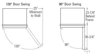
Allow 25" minimum clearance for a full to Wall 130° door swing. Allow 15" for pan removal.
