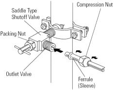
**NOTE:** It is best to install the valve into a vertical water pipe. If you install the valve into a horizontal water pipe, make the connection at the top or side to avoid drawing off any sediment from the water pipe.
