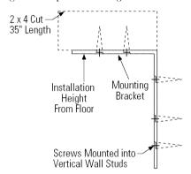
• Secure the bracket with wood block to the back wall so that it is 84" (or your installation height) from the finished floor.
