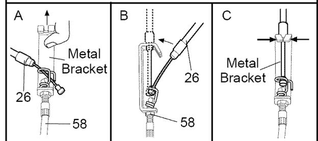
4. While a second person holds the Console (6) near the Console Bracket (45), connect the Extension Wire (62) to the console wire. Make sure the slack Resistance Cable (26) is pulled out of the Upright (3).
