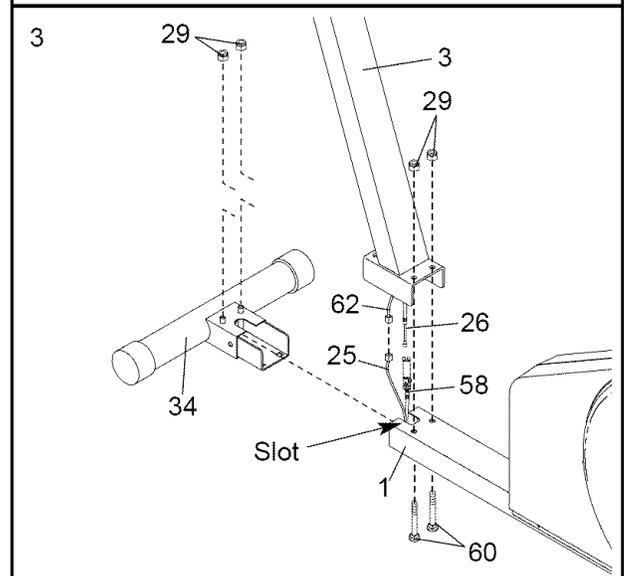
While a second person holds the Upright (3) near the Frame (1), connect the Reed Switch Wire (25) to the Extension Wire (62). Next, connect the Resistance Cable (26) to the Lower Cable (58) in the following way:
