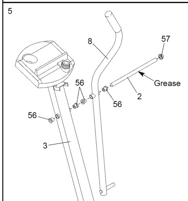
6. Slide the other Handlebar (8) onto the Pivot Axle (2). Secure the Handlebars to the Upright (3) by tapping a 5/8" Axle Cap (57) onto the end of the Pivot Axle.
