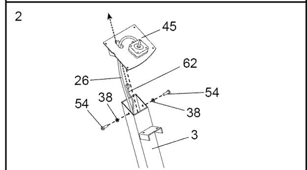
Attach the Console Bracket (45) to the Upright (3) with two M6 x 16mm Button Screws (54) and two M6 Split Washers (38). **Make sure not to pinch the Resistance Cable (26) or the Extension Wire (62).**
