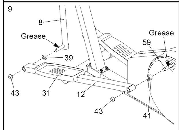
Attach the other Pedal Arm (not shown) to the right side of the elliptical in the same way.
