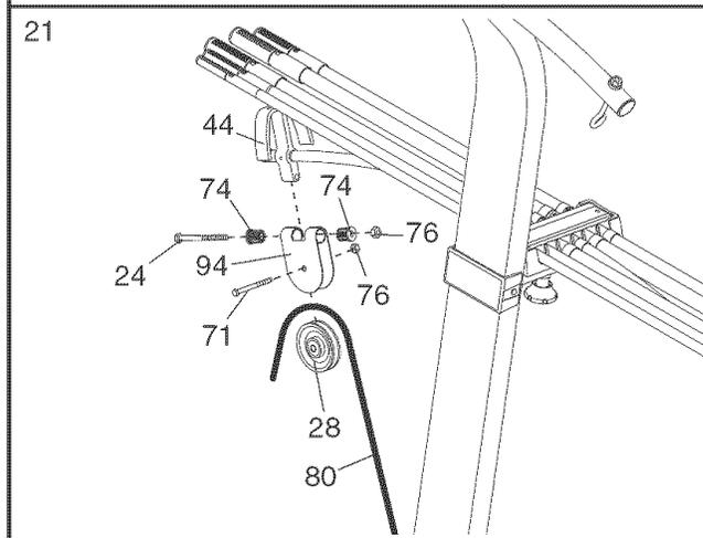
Wrap the Long Cable (80) over a 90mm Pulley (28). Attach the Pulley inside of the Pulley Housing (94) with an M10 x 42mm Button Bolt (71) and an M10 Nylon Locknut (76).
