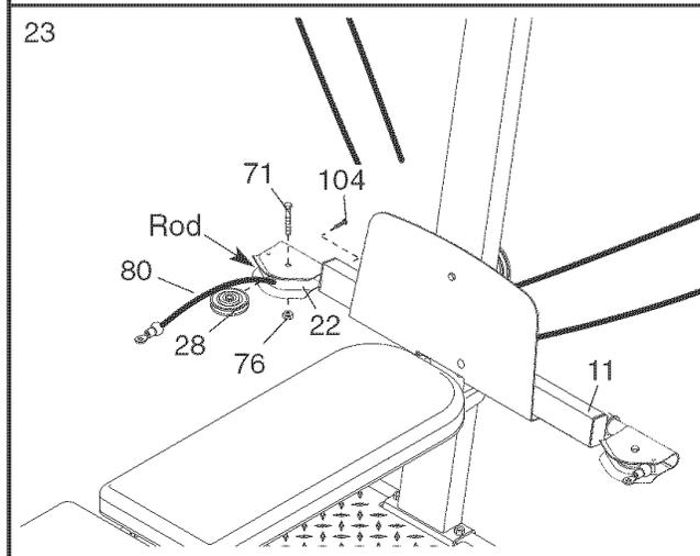
Insert the end of the Long Cable (80) through the welded tube on the indicated end of the Cross Tube (11) and then through the remaining Swivel Arm (22). **Make sure the Cable is on the indicated side of the welded rod in the Swivel Arm.**
