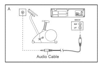
B. Plug one end of a 1/8" to RCA stereo audio cable (available at electronics stores) into the jack beneath the console. Plug the other end of the cable into an RCA Y-adapter (available at electronics stores). Next, remove the wire that is currently plugged into the AUDIO OUT jack on your VCR and plug the wire into the unused side of the Y-adapter. Plug the Y-adapter into the AUDIO OUT jack on your VCR.
