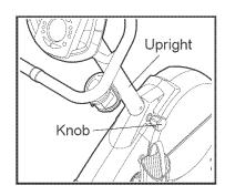
is not loosened enough, it may scratch the upright). Next, pull the knob, slide the upright to the desired height, and then release the knob. Move the upright up and down slightly until it locks into position. Then, turn the knob clockwise until it is tight. IMPORTANT: After you adjust the upright, make sure that your knees will not touch the handgrip pulse sensor when you pedal.
