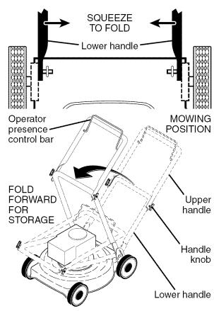
2 POSITION / "ADJUSTABLE" HANDLES When setting you handles up from the storage position, the lower handle will automatically lock into mowing position.
