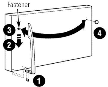
**Reinstalling the handle:** Attach the handle to the right side of the door.
