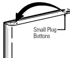
Move the large plug button from the left edge of the door and insert it into the hole on the opposite side.
