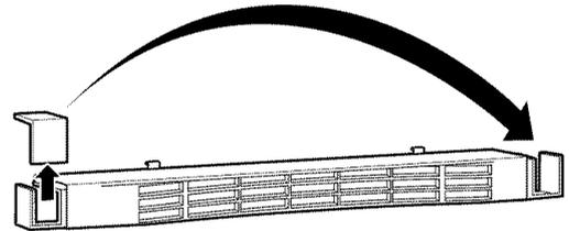
Using a socket driver, move the bottom hinge bracket from the right side to the left side.
