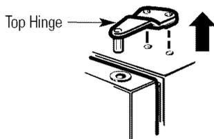
Remove the tape and tilt the door away from the cabinet. Lift it off the center hinge pin.
