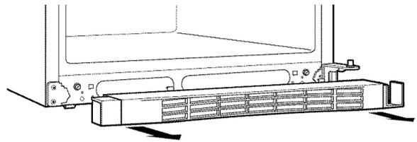
Remove the insert at the top left side of the base grille and install it on the right side. You must pull up on the insert to remove and snap down to replace.
