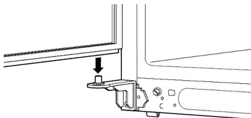
Straighten the door and line it up with the center hinge bracket.
