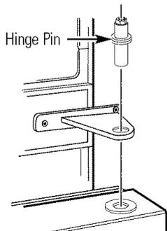
Remove the tape and tilt the door away from the cabinet. Lift the door straight off the bottom hinge bracket.
