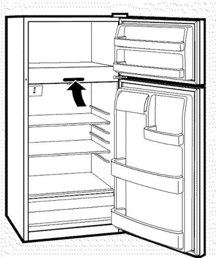
Initially, set the refrigerator control at **5** and the freezer control at **5** and allow 12–24 hours for the temperature to stabilize.
