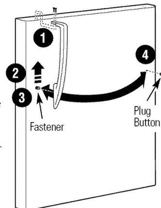
**After removing the handle:** Move the small plug buttons from the top right side of the door top and insert them into the holes on the opposite side.
