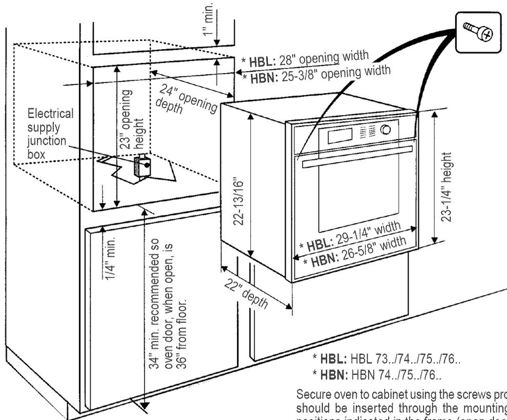
Secure oven to cabinet using the screws provided. Screws should be inserted through the mounting holes in the positions indicated in the frame (open door to see frame and mounting holes). Do not overtighten screws.
