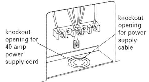
**8.** Depending on your electrical supply, make the four-wire or three-wire connection to the range following the "Power supply cord method" or "Direct wire method" instructions for copper wire or aluminum wire depending on the connection needed.
