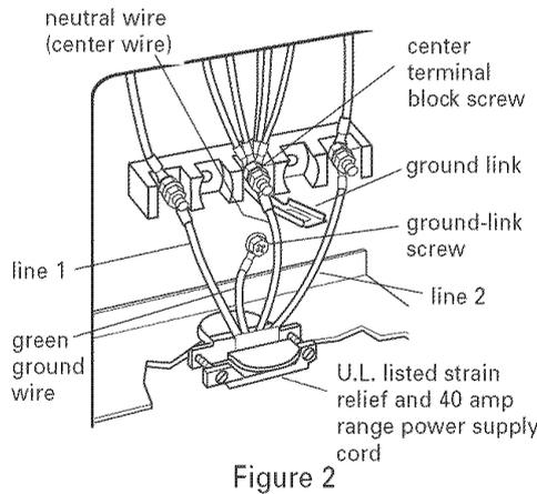
Use this method for mobile homes and whenever four-wire installation is required.
