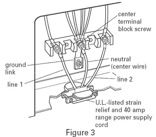
Use this method only if local codes permit connecting cabinet-ground conductor to neutral wire of power supply cord.
