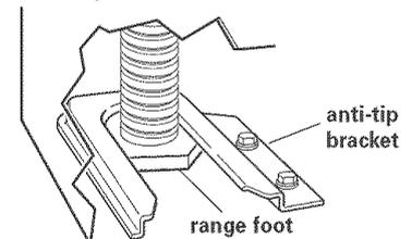
3. Make sure the anti-tip bracket is installed:
