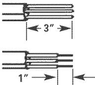
4. Strip outer covering back 3 inches from end, exposing wires. Strip the insulation back 1 inch from the end of each wire.
