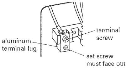
7. **IMPORTANT:** the aluminum terminal lugs must be assembled to the terminal posts with the set screws facing out as shown.
