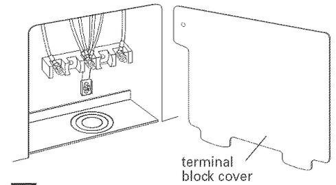
**7.** Remove the terminal block cover located on the back of range.
