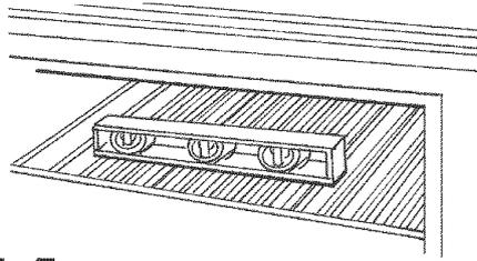
**14.** Place rack in oven. Place level on rack, first side to side; then front to back.
