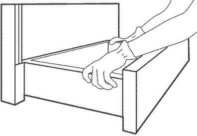
**11.** Pull drawer open to first stop position. Lift front of drawer to clear white wheels in drawer guides. Remove drawer and set it aside on a protected surface.
