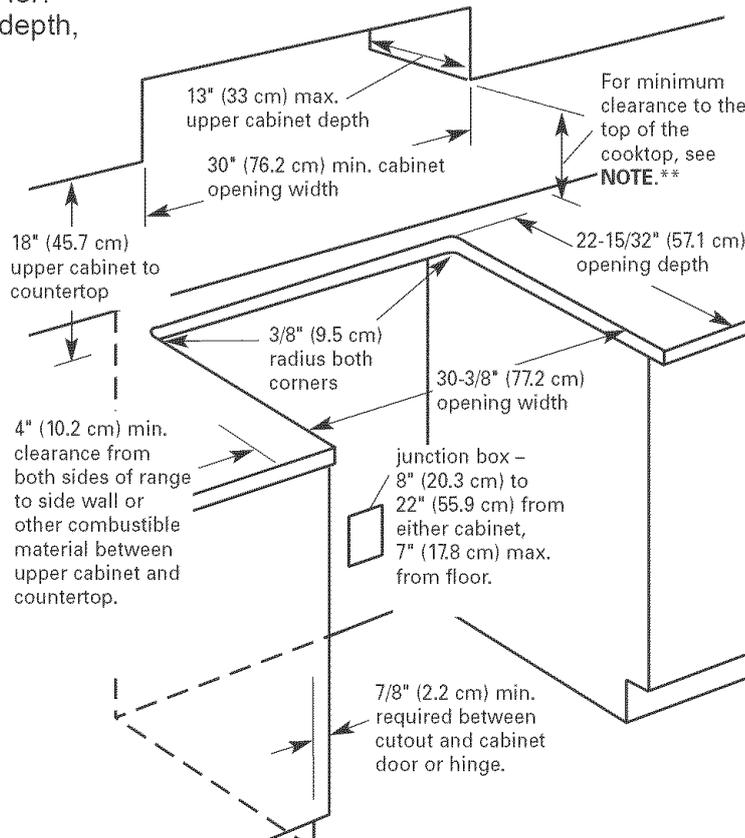
**\*\*NOTE:** 24" min. when bottom of wood or metal cabinet is protected by not less than 1/4" flame retardant millboard covered with not less than No. 28 MSG sheet steel, 0.015" stainless steel, 0.024" aluminum or 0.020" copper.
