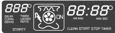
Check the operation of the oven element. Press the "BAKE" button. "350°" will appear in the temperature display. The ON, Bake Element, Outer Broil Element and Oven Cavity symbols will light up in the display. Press the "START/ENTER" button.
