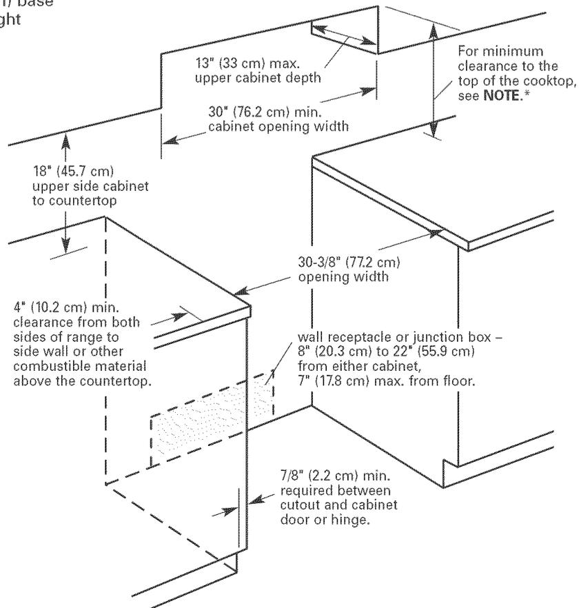
**\*NOTE:** 24" (61 cm) min. when bottom of wood or metal cabinet is protected by not less than 1/4" (6.4 mm) flame retardant millboard covered with not less than No. 28 MSG sheet steel, 0.015" (0.4 mm) stainless steel, 0.024" (0.6 mm) aluminum or 0.020" (0.5 mm) copper.
