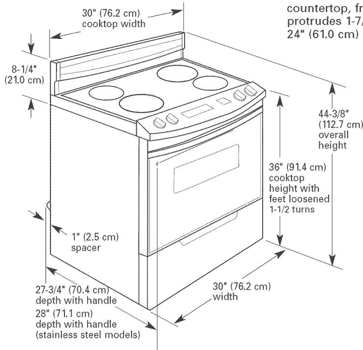
When installed in a 24" (61.0 cm) base cabinet with 25" (63.5 cm) countertop, front of oven door protrudes 1-7/8" (4.8 cm) beyond 24" (61.0 cm) base cabinet.
