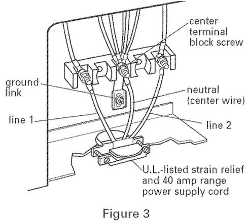
Use this method only if local codes permit connecting cabinet-ground conductor to neutral wire of power supply cord.
