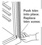
Slide top end of each trim upward onto range side rails. Push each trim into place at bottom of trim. Use screws to attach each trim to range. Take care not to scratch other surfaces with ends of trim.
