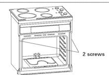
Important: Securely fasten range to cabinet using the two screws provided. Insert the screws through holes in mounting rails. Do Not overtighten screws.
