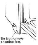
range. The shipping feet will protect the lower range trim until range is inserted into
