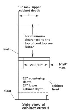
\*Note: 24" min. when bottom of wood or metal cabinet is protected by not less than 1/4" flame retardant millboard covered with not less than No. 28 MSG sheet steel, 0.015" stainless steel, 0.024" aluminum or 0.020" copper.
