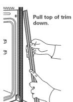
Remove trim screws attaching right and left side trim to range. Grasp the bottom end of trim and pull away from range. Slide top end of trim downward to remove trim from range. Take care not to scratch other surfaces with ends of trim. Set trim and screws aside on protected surface.
