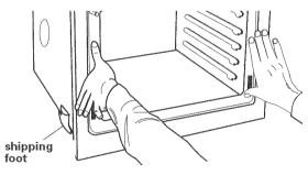
Push against seal area of front frame to push range into cabinet until shipping feet almost contact cabinet. Use a Phillips screwdriver to remove screws attaching shipping feet. Remove and discard shipping feet.
