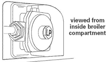
**2.** Open broiler drawer and remove broiler pan. The pressure regulator is located in the back right hand corner of the broiler compartment.
