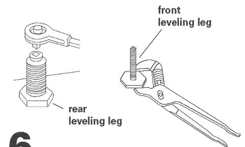
**6.** Remove cardboard shipping base from under range. Open broiler door. Use a 3/8" drive ratchet to lower rear leveling legs one-half turn. Use slip-joint pliers to lower front leveling legs one-half turn.
