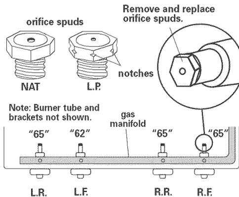
d. Locate L.P. gas orifice spuds for top burners in literature package included with the range. Three L.P. gas spuds are stamped "65" and one "62". Remove Natural gas orifice spuds using a 3/8" combination wrench. Install L.P. gas orifice spuds in locations shown to replace the Natural gas orifice spuds. Note: Depending on model, the range cooktop may be equipped with 4 standard burners or 3 standard burners and 1 power burner. Spud size/location remain the same.
