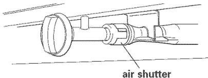
**c.** Adjust the air shutter by hand as needed. Close the air shutter to decrease the amount of air to the flame. Open the air shutter to increase the amount of air to the flame.
