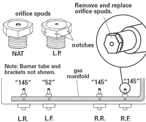
**d.** Locate Natural gas orifice spuds for top burners in literature package included with the range. Three Natural gas spuds are stamped "145" and one "52". Remove Natural gas orifice spuds using a 3/8" combination wrench. Install Natural gas orifice spuds in locations shown to replace the L.P. gas orifice spuds. Note: Depending on model, the range cooktop may be equipped with 4 standard burners or 3 standard burners and 1 power burner. Spud size/location remain the same.
