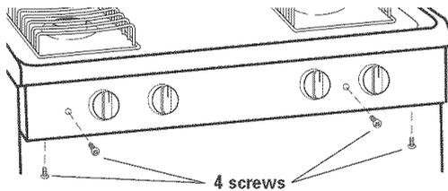
**a.** Remove control knobs and 4 screws that attach control panel to range cabinet. Pull control panel forward to remove. Set panel, screws and knobs aside.
