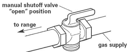
**Shutoff valve:** The supply line must be equipped with a manual shutoff valve. This valve should be located in the same room as the range and should be in a location that allows ease of opening and closing. The valve is for turning on or shutting off gas to the range. **Do Not block access to shutoff valve.**
