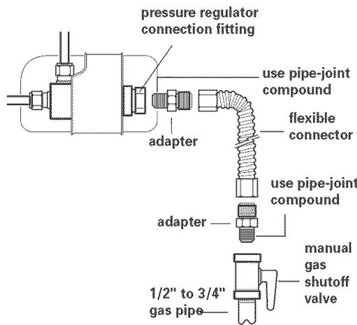
A 1/2" male pipe thread is needed for connection to pressure regulator female pipe threads.
