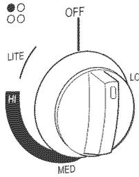
**17.** Push in and turn each surface unit control knob to “LITE” position. The flame should light within 4 seconds. Turn control knob to “HI” position after burner lights.
