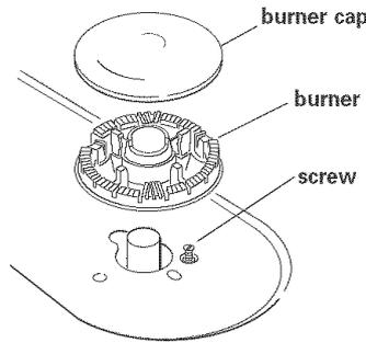
**4.** Remove burner grates, burner caps, burners and screws. Lift cooktop. Note: There is no cooktop support rod.
