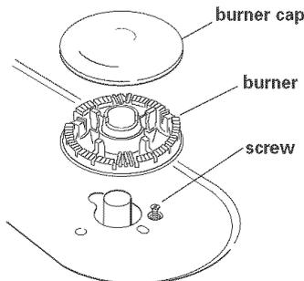
**4.** Remove burner grates, burner caps, burners and screws. Lift cooktop. Note: There is no cooktop support rod.
