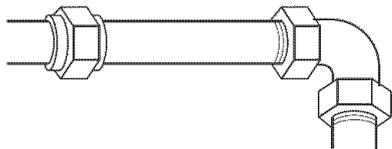
**Rigid pipe connection:** Requires a combination of pipe fittings to obtain an in-line connection to the range. All strains must be removed from the supply and fuel lines so range will be level and in line.
