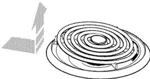
2. Pull the coil element straight away from the receptacle.
