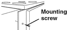
Making sure the mounting screws are installed:
