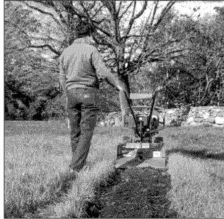
Figure 4-4: Guide tiller with one hand.
