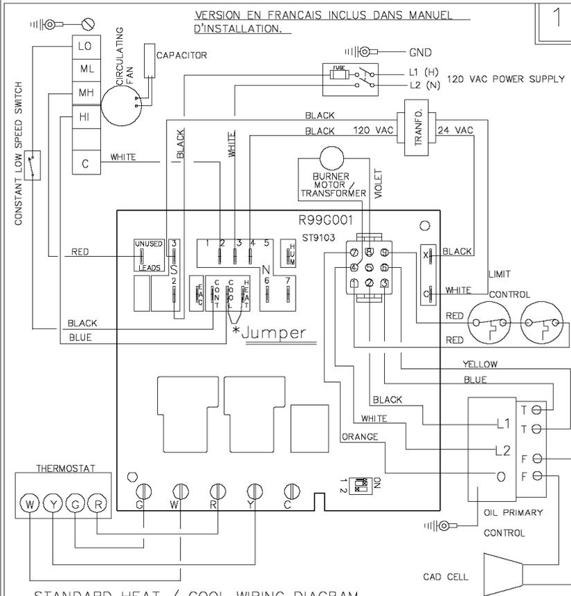
STANDARD HEAT / COOL WIRING DIAGRAM WITH ST9103 ELECTRONIC FAN TIMER
