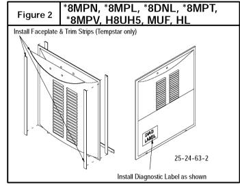
Place one Diagnostic Label on the bottom left corner of the sound shield installed on the backside of the door.
