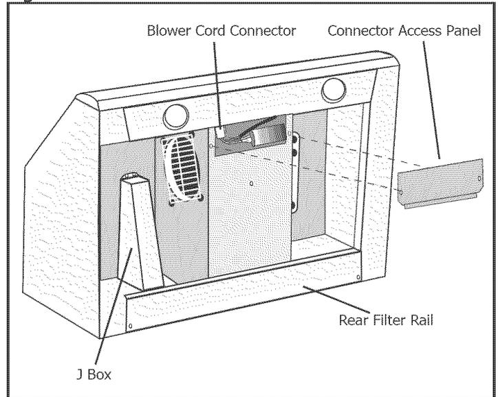
Figure 2 - DAH95 models with internal blower
