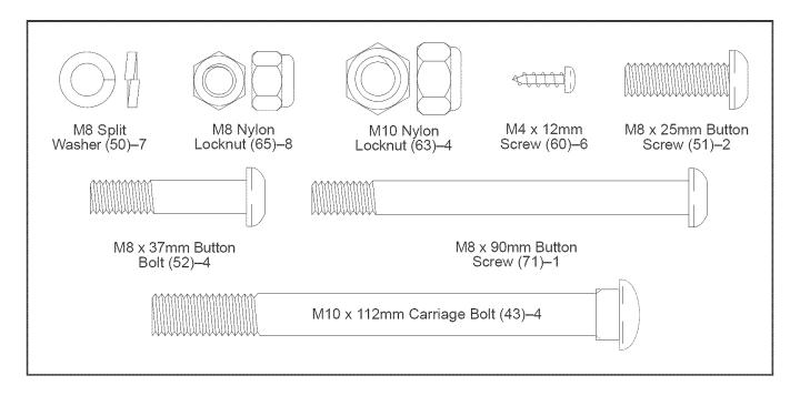
1. Attach the Rear Stabilizer (16) to the Rear Stabilizer Leg (41) with two M10 x 112mm Carriage Bolts (43) and two M10 Nylon Locknuts (63).
