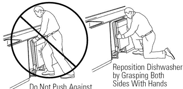
Do Not Push Against Front Door Panel With Knee. Damage to The Door Panel Will Occur.
