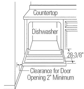
**CLEARANCES:** When installed into a corner, allow 2" min. clearance between dishwasher and adjacent cabinet, wall or other appliances. Allow 28-3/8" min. clearance from the front of the dishwasher for door opening (Figure B).
