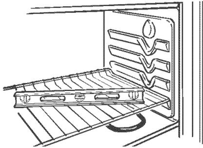
Install the oven shelves (see use and care section for instructions). Put a spirit level or a glass measuring cup partially filled with water on one of the oven shelves.
