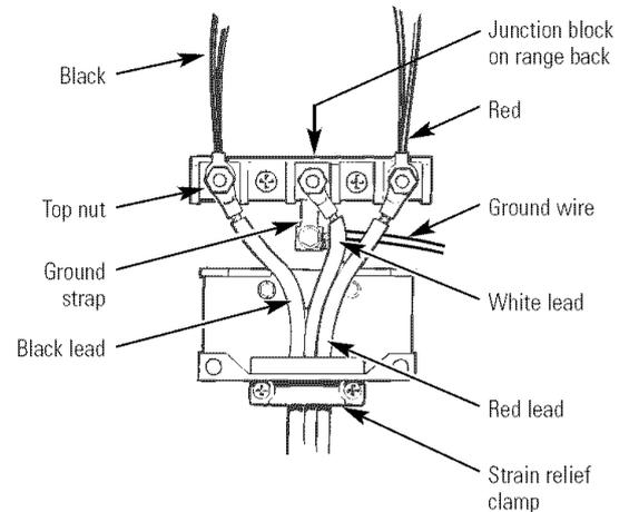
Then loosen the screw from the ground strap and fasten a #10 copper wire to the range. Secure the other end of the wire to a grounded cold water pipe or use another approved grounding method.
