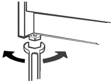
Use a 1 $\frac{3}{8}$ " open end wrench or an adjustable wrench to back out the four leveling legs two or three turns each. Now use the wrench to adjust the leveling legs until the range is level.
