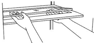
3. Replace back of meat drawer cover frame into supports or slides on side walls of the refrigerator and lower or slide the front of the cover frame into place.
