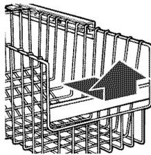
3. Replace the basket or bin by positioning it on the side wall guide rails. Lift the basket or bin front slightly while pushing it past the guide rail stops and slide basket or bin in the rest of the way.
