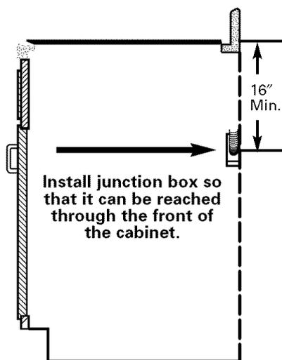
**▲ IMPORTANT:** The junction box must be located where it will allow considerable slack in the conduit for serviceability.
