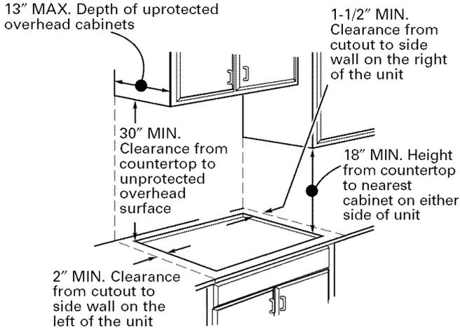
If a 30" clearance between the cooking surface and overhead combustible materials or metal cabinets cannot be maintained, a minimum clearance of 24" is required and the underside of the cabinets above the cooktop must be protected with not less than 1/4" insulating millboard covered with sheet metal not less than 0.0122" thick.
