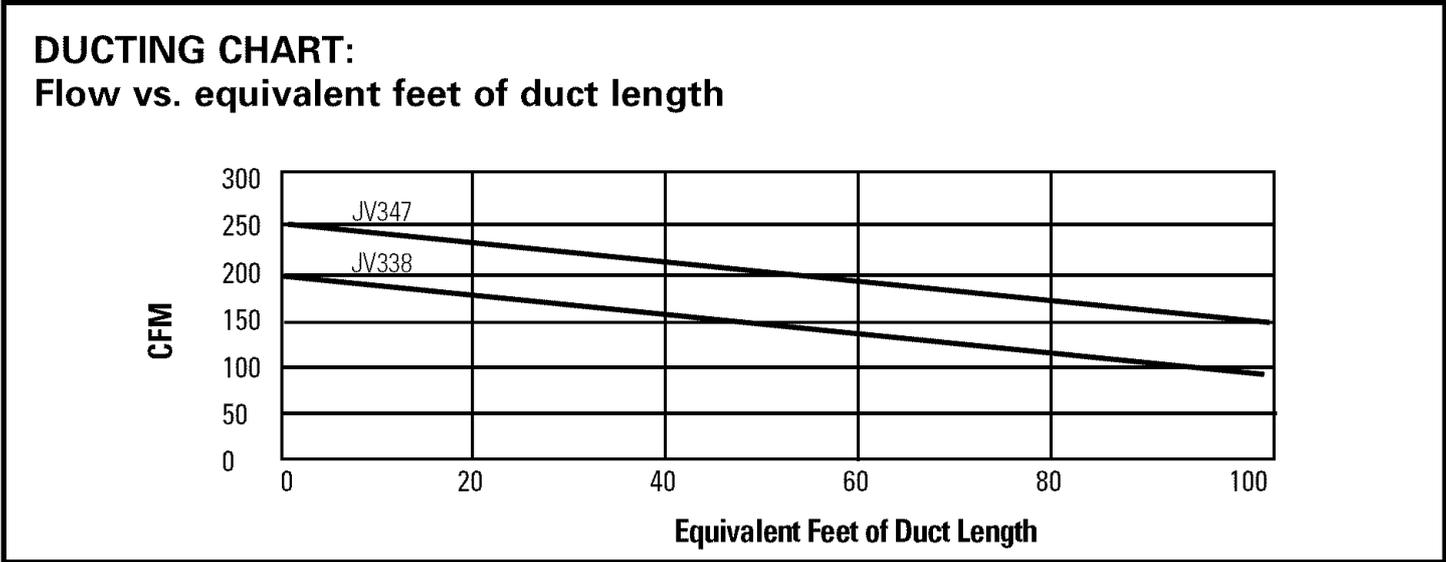
**MAXIMUM DUCT LENGTH:** For satisfactory air movement, the total duct length of a 3/4" x 10" rectangular, 6" or 7" diameter round duct **should not exceed 65 equivalent feet.**
