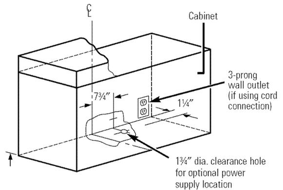
**NOTE:** If using optional Power Cord Kit JXHC1, feed the power cord through the hole in the top cabinet while raising the hood. Loop any excess length of cord and tie away with a suitable tape or tie.
