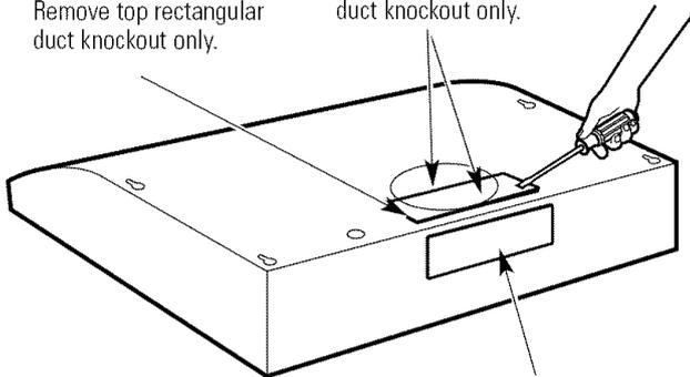
**3 1/4" x 10" Rectangular horizontal discharge.** Remove rear rectangular duct knockout only.
