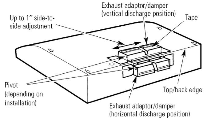
**NOTE:** The exhaust adaptor/damper can be installed up to 1 inch on either side of the hood center to accommodate off-center ductwork. In extreme off-center installations, one end of the duct connector may need to be trimmed to clear the electrical cable clamp.
