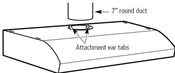
Use **duct tape** to make joints secure and air tight.
