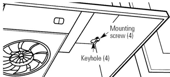
**NOTE:** DO NOT PUSH ON FAN BLADE. Pushing on the blade may cause it to interfere with other hood parts.
