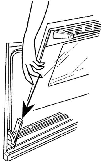
**The oven door is heavy. You may need help lifting the door high enough to slide it down onto the hinges. Do not lift the door by the handle.**
