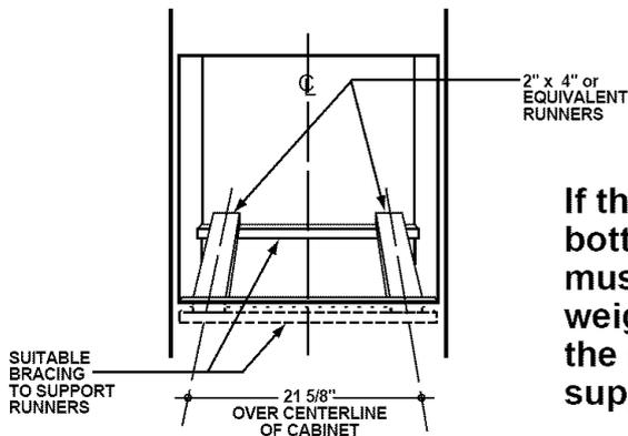
If the cabinet does not have a solid bottom, then two braces or runners must be installed to support the weight of the oven. For single ovens the runners and braces must support 150 pounds.
