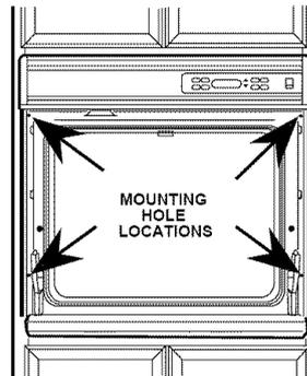
The screws must be a minimum of 1/4" from the front of the cutout.
