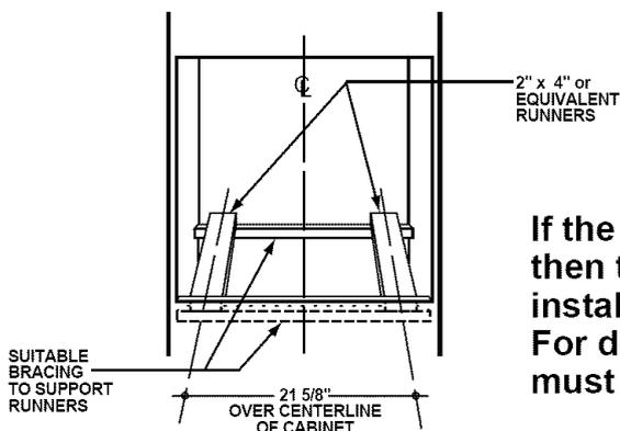
If the cabinet does not have a solid bottom, then two braces and runners must be installed to support the weight of the oven. For double ovens the runners and braces must support 275 pounds.
