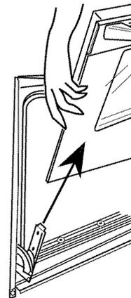
**NOTE:**The oven door is very heavy. Be sure you have a firm grip before lifting the oven door off the hinges. Use caution once the door is removed. Do not lay the door on its handle. This could cause dents or scratches
