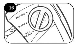
For dry debris pickup, turn the dial to the DRY VAC position. In this position, the brushes will not rotate and are raised off the floor surface.
