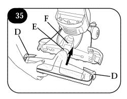
To replace nozzle, make sure latches (D) are out.
