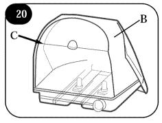
Pour cleaning concentrate into tank (B). Fill tank to fill line (C) (1 quart) with warm water.
