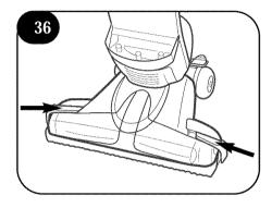
While holding nozzle in place, slide latches inward to lock in place.
