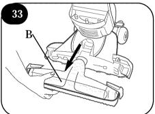
Remove nozzle (B) by pulling straight out.
