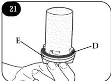
If rubber ring (D) on cap has become dislodged, reposition it with uneven side against ledge (E) as shown.
