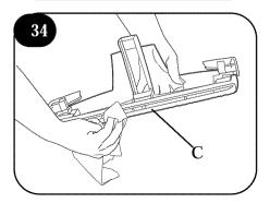
Rinse nozzle under running water. Remove debris from squeegee (C) and wipe with a damp cloth.
