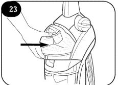
Slide tank straight into position until latch snaps in place.
