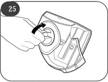
Slide tank straight into position until latch snaps in place.
