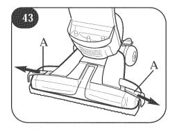
Remove nozzle (B) by pulling straight out.
