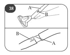
The handle must be in the upright position in order to get cleaning solution through the hose.
