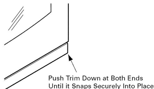
**CAUTION:** Be sure you do not tip the oven forward during installation or you may bend the bottom trim. The bottom trim provides an opening for cooling air to enter the cabinet. This opening should never be blocked.
