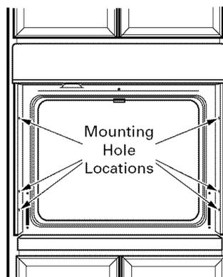
The screws must be a minimum of 1/4" from the front of the cutout. (Door not shown in this view.)
