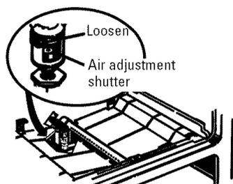
The shutter for the bottom (oven) burner is near the back wall behind the warming drawer. Remove the drawer. See the *Care and cleaning of the range* section.
