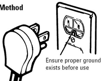
The power cord of this appliance is equipped with a 3-prong (grounding) plug which mates with a standard 3-prong grounding wall receptacle to minimize the possibility of electric shock hazard from this appliance.
