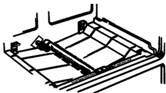
To determine if the bottom burner flames are burning properly, remove the oven bottom. Flames should have approximately 1" blue cones and, if range is supplied with natural gas, should burn with no yellow tipping. (With most LP gas, small yellow tips at the end of outer cones are normal.) Flames should not lift off burner ports. If lifting is observed, gradually reduce air shutter opening until flames are stabilized.
