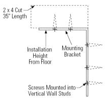
Secure the bracket with wood block to the back wall so that it is 84" (or your installation height) from the finished floor.
