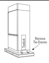
• Remove the four 7/16" bolts securing the straps to the skid.
