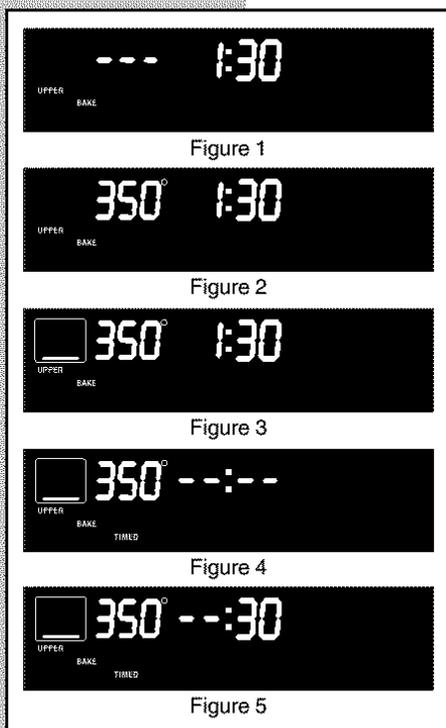
To program the oven for a delayed **BAKE** start time and to shut off automatically (example for upper oven baking at 350°F, starting at 5:30 for 30 minutes):
