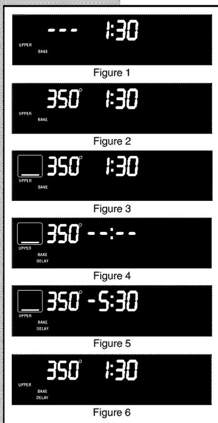
To program the upper oven for a **DELAYED BAKE** start time and to shut off **MANUALLY** (example for upper oven baking at 350°F, starting at 5:30):
