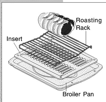
When preparing meats for convection roasting, use the broiler pan and insert along with the roasting rack. The broiler pan will catch grease spills and the insert will help prevent spatters. The roasting rack will allow the heat to circulate around the meat.
