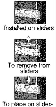
Pull oven rack forward and lift it up off the oven rack slider.
