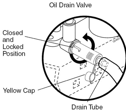
3. Unlock drain valve by pushing inward slightly and turning counterclockwise.
