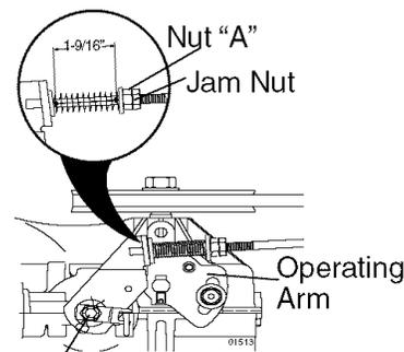
Do not touch this nut. If further brake adjustment is necessary contact a Sears or other qualified service center.
