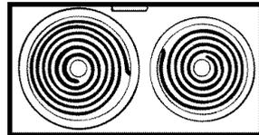
This module has one 6" and one 8" coil surface unit. The surface units and drip pans are removable for cleaning.
