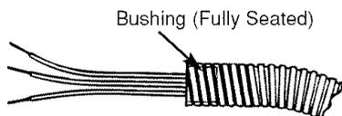
Thread the leads through an anti-short bushing and firmly seat the bushing in the end of the conduit.
