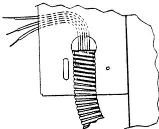
Lay the conduit against the side of the wire compartment.
