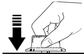
Push the knob in and turn in either direction to the heat setting desired.
