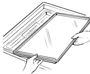
4. Place the griddle plate on the reflector pan over the heating element. The plate should be seated properly on the reflector pan with the griddle's drain holes at the front.
