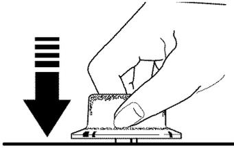
**The control knob must be pushed in to turn;** this prevents the heating element from being turned on accidentally. Push the knob in only when it is in the OFF position. When the knob is in any other position, it can be turned without pushing it in.
