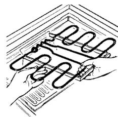
3. Make sure all controls are turned to OFF. Hold the heating element with the plug facing the side of the cooktop and level with the surface. Insert the plug into the cooktop outlet as far as it will go. (Do not force.) The heating element support should rest on the ledge of the reflector pan.
