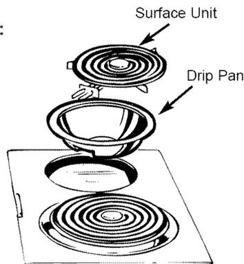
**Repeated lifting of the surface unit more than 1 inch above the drip pan can permanently damage the receptacle.**
