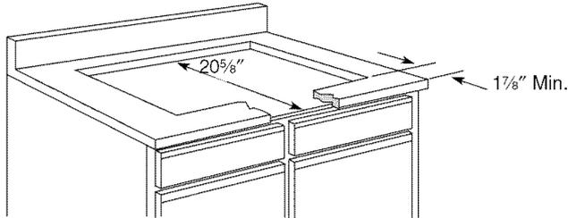
A  $1\frac{1}{2}$ " wide flat area is required around the edge of opening for support of the unit. The cooktop unit must be level and sit squarely into countertop opening.
