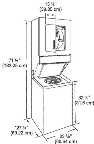
\*Most installations require a minimum 5 1/2" (14 cm) clearance behind the dryer for the exhaust vent with elbow. See "Venting Requirements."
