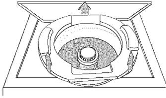
**NOTE:** Keep the foam ring and use it when transporting your washer/dryer. This packing material is used to keep the washer tub stable during transport.
