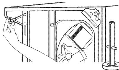
2. Check adjustability of rear legs by pushing in one leg. The other leg should come out. Check both legs. If they do not move freely, repeat Step 1.
