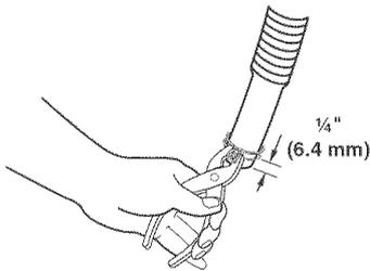
4. Open clamp. Twist hose back and forth while pushing onto drain connector on the side of the washer/dryer. Continue until hose contacts the ribbed stops on the cabinet.
