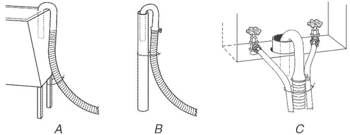
If the water faucets and the drain standpipe are recessed, put the hooked end of the drain hose in the standpipe. Tightly wrap the plastic strap around the water inlet hoses and the drain hose (C above).
