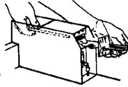
For dryers using coin slides, use adapter kit supplied with dryer. Replace the meter case service door. Put the coin vault with lock and key the meter case opening.
