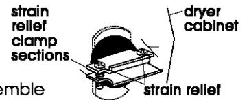
**3. Assemble 3/4" U.L.-listed strain relief (U.L. marking on strain relief) into the hole below terminal block opening. Tighten strain relief screws just enough to hold the two clamp sections together. Install power supply cord/cable through the strain relief.**
