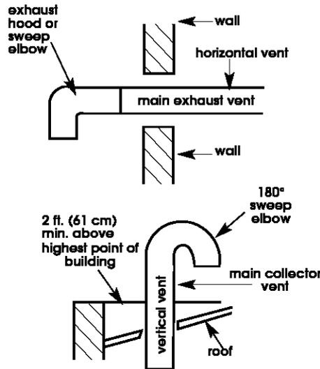
**Do Not** install screening or cap over end of vent.
