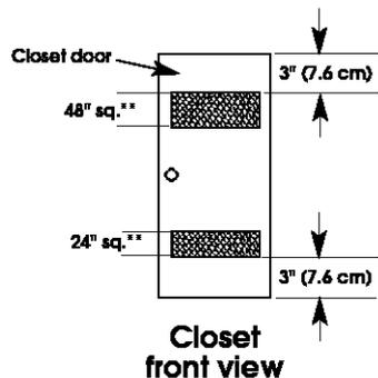
\* Additional clearances for wall, door and floor moldings may be required or if external exhaust elbow is used.
