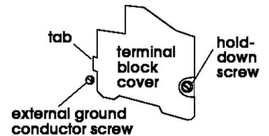
**2. Remove hold-down screw and terminal block cover.**
