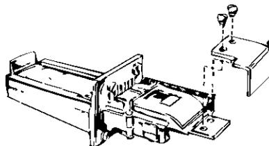
**6.** Open control panel and rest it on the bottom edge of the opening. Attach slide extension (with flange pointing down) to one of the coin-slide mechanisms. Insert the coin-slide mechanism through the opening to left of the control panel.
