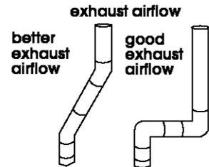
**Four-inch (10.2 cm) metal exhaust vent** is required. Plan installation to use the fewest number of elbows and turns.
