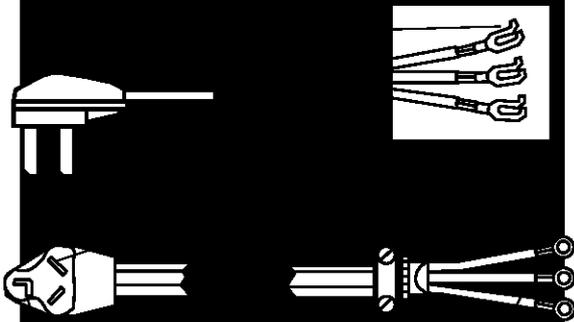
Three-wire power supply cord must have three, No.-10 copper wires and match a three-wire receptacle of NEMA Type 10-30R.
