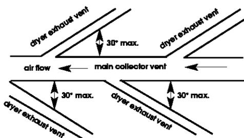
**Back-draft Damper Kits**, Part No. 3391910, are available from your Whirlpool dealer and should be installed in each dryer's exhaust vent to prevent exhausted air from returning into the dryers and to keep the exhaust in balance within the main exhaust vent. Unobstructed air openings are required.
