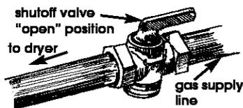
**F.** The supply line shall be equipped with a shutoff valve installed within 6 ft. (1.8 m) of dryer in accordance with the National Fuel Gas Code, ANSI Z223.1 — latest edition\*. This valve should be located in the same room as the dryer and should be in a location that allows ease of opening and closing. Do Not block access to the shutoff valve.
