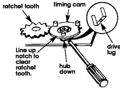
4. Insert a narrow, flat-blade screwdriver under the timing cam near the clock shaft. Gently lift cam straight up and off shaft making sure that the "V"-shaped notch clears the ratchet tooth.
