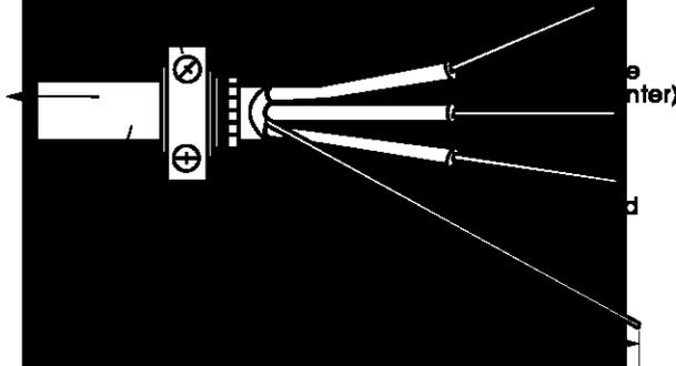
Strip 5" (12.7 cm) of outer covering from end of cable. Leave bare ground wire at 5 inches (12.7 cm). Cut 1-1/2" (3.8 cm) from 3 remaining wires. Strip insulation back 1 inch (2.5 cm).
