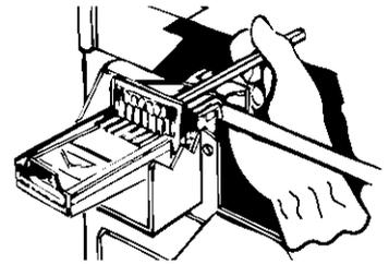
**7.** Secure coin slide mechanism from inside the control panel using the 3/16" bolt and washer included with the slide mechanism. Install coin box.
