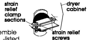
3. Assemble 3/4" U.L.-listed strain relief (U.L. marking on strain relief) into the hole below terminal block opening. Tighten strain relief screws just enough to hold the two clamp sections together. Install power supply cord/cable through the strain relief.
