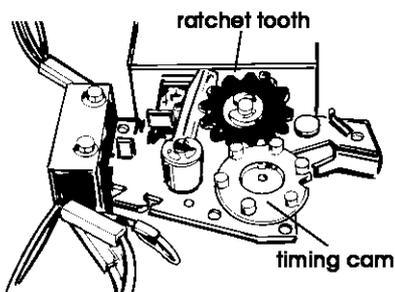
3. Turn the timing cam by hand until the "V"-shaped notch lines up below the ratchet tooth.
