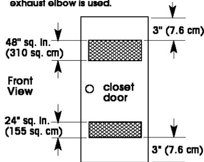
Opening is minimum for closet door. Louvered door with equivalent air openings is acceptable. Companion appliance spacing should be considered.
