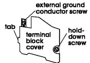
2. Remove hold-down screw and terminal block cover.
