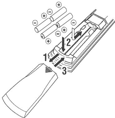
**1** Press the ▼ part and slide the battery compartment cover off.
