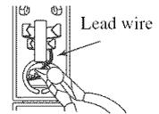
**4** Insert the cable wire into the slot, and clamp it with pliers.
