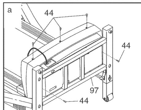
With the help of a second person, carefully raise the Upright Base (97) as shown. Carefully pivot the Hood (113) off.
